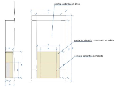
DETTAGLIO ARREDO SU MISURA IN LEGNO NELLA NICCHIA DELL'ABSIDE PER MASCHERARE COLLETTORE - SCALA 1:20
